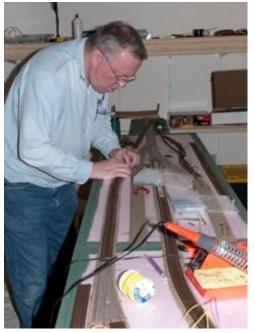
40 feet of track-work that included seven turnouts. Code 83 rail was laid using Paul's experienced personal skillset. While Paul laid rail, Roger drilled holes, cut and installed feeder wire on either side of the turnouts and extensions (about two dozen feed wires). Paul demonstrated his technique of soldering to light rail. Roger parroted the soldering technique well enough and at 1:30AM Saturday morning we finished.
